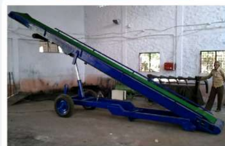
LOW - INTAKE CONVEYOR
